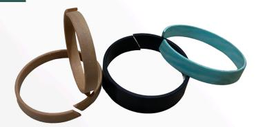
Guide belts, also known as guide rings, are essential components in hydraulic and pneumatic cylinders. These belts are positioned around the piston or rod to provide a smooth, low-friction surface that guides the movement of these parts within the cylinder bore. By maintaining proper alignment and preventing metal-to-metal contact, they minimize the risk of scratches or damage to the barrel and rod of the cylinder.
